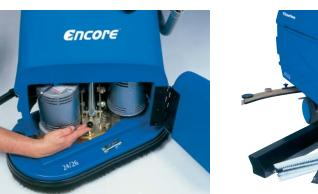
Changing the scrub deck width on the Encore 24/26 from 24 to 26 inches is simply a matter of lifting the black knob and rotating the deck.
