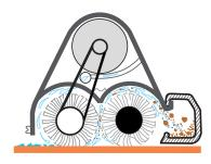
Choose disk scrubbing (above) or cylindrical scrubbing (below) with debris pick up to meet facility's cleaning needs.
