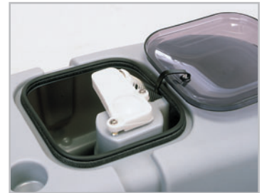
The recovery tank is fitted with a float system that shuts off vacuum air flow when the tank is full to prevent overflow. Large opening permits easy, unobstructed cleanout.
