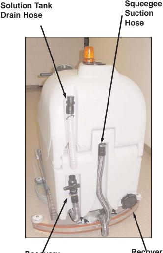
Recovery Tank Discharge Hose and Valve Recovery Tank Clean-Out
