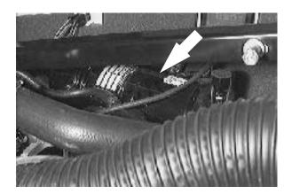
Install the dust cap on the air filter housing with the arrows pointing up.
