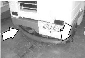
If the machine has the optional rear tie down brackets, attach the winching chains to them.
