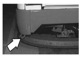
Turn the bypass valve 90° from the normal position before winching the machine onto the truck or trailer. See *PUSHING OR TOWING THE MACHINE* section of this manual. Make sure the machine is centered.
