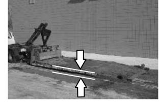
To winch the machine onto the truck or trailer, attach the winching chains in the holes at the bottom of the rear bumper.
