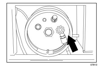
Open the tank service valve slowly and check for leaks. Close the service valve immediately if an LPG leak is found, and tell the appropriate personnel.
