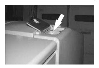
ES™ mode: Lift up the operator seat. Remove the detergent tank lid and pour the required amount of detergent into the tank. Put the lid back on the detergent tank and lower the operator seat.
