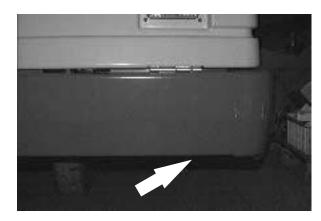
The rear jacking locations are the two rear corners of the machine frame.
