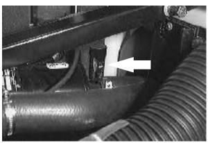
☐ Check the engine oil level.
