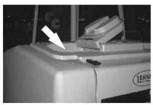
9. Remove the large drain cap and flush out the bottom on the recovery tank.
