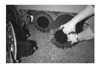
**Polypropylene side scrub brush** - A general-purpose brush with stiff bristles for aggressive action on slightly compacted soilage. Works well on concrete, wood, and tile surfaces.
