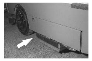
☐ Check the engine air filter indicator.
