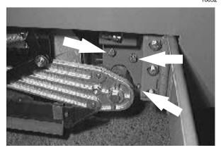
The brush patterns should be the same width. If one is narrower then the other, the scrub head needs to be leveled from front to rear.
