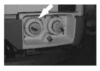
10. ES™ mode: Clean the ES™ filter. If the filter can't be rinsed off through the right recovery tank fill opening, the filter can be removed from the recovery tank by disconnecting the ES™ pump wire and solution hose, and unscrewing the ES™ pump cap from the recovery tank.
