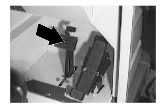
3. Select the (Idle) position with the engine speed switch.
