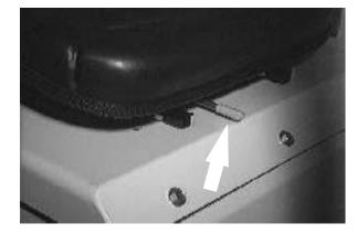
Lift: Pull up on the seat mounting plate until the seat mount locks up.
