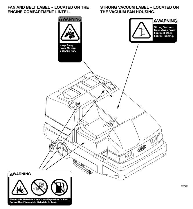
FLAMMABLE MATERIALS LABEL - LOCATED NEXT TO THE SOLUTION TANK COVERS AND ON THE DETERGENT TANK.
