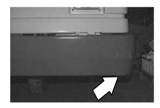
The rear tie down locations are in the holes at the bottom of the rear bumper. If the machine has the optional rear tie down brackets, use them to tie down the machine.
