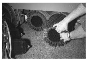
11. Line up the drive end of the new or rotated brushes with the brush drive plugs. The cylindrical scrub brushes must be installed with the V-patterns on the brushes pointing towards each other. Slide the brushes onto the brush drive plugs.
