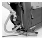
Rear solution fill port permits filling solution tank while emptying the recovery tank.
