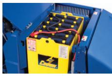
800 AH battery on battery model can be quickly changed with optional roll on roll off system.
