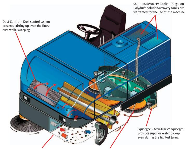
Sweeping System - True sweeping system with variable dump hopper picks up dirt and debris before scrubbing
