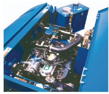
Models available with Ford EFI gas, LP or Mitsubishi diesel engines to meet your power needs. Engines meet EPA requirements through 2007.
